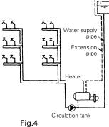
In large-scale hot water supply system, the piping is long and complicated, so the piping resistance increases and the natural circulation of hot water becomes impossible. Therefore, it is necessary to forcibly circulate the hot water with a pump. It is used for its forced circulation purpose.
