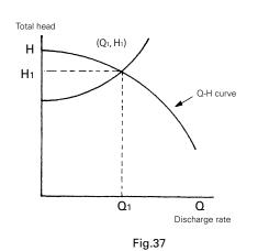
If the total pump head required to deliver the discharge rate Q1 at the site is H1, it is necessary to select the pump whose Q-H curves passes this (Q1, H1).
