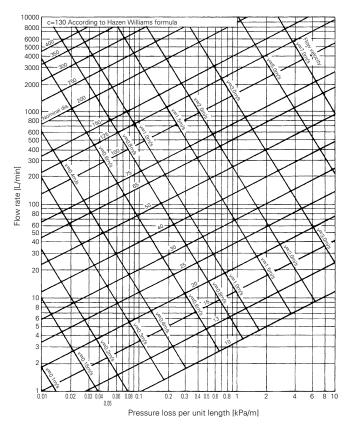
Fig. 24. Rigid vinyl chloride pipe flow rate diagram (SHASE-S 206-2009)
