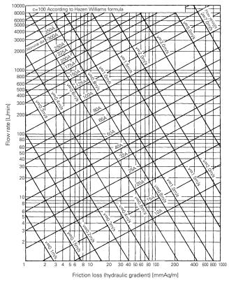
Fig. 22. Carbon steel pipes for ordinary piping (JIS G 3452) flow rate diagram (HAS-S 206-1982)
