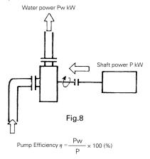
Pump efficiency is the rate at which mechanical energy, or shaft power, P, can be converted to water power, Pw. The higher this value, the better the efficiency. For example, if the shaft power P=10kW and the water power Pw=6kW, the pump efficiency  $\eta$  (%)
