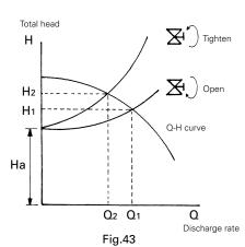
Using this principle, the water volume of the pump is controlled by a valve. As described above, the pump operating point is determined by the intersection of the Q-H curve and the resistance curve. However, by changing the resistance curve by valve operation, the operating point can be changed to obtain the required discharge amount.
