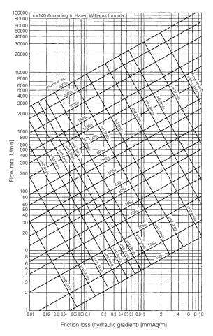
Fig. 23. Stainless steel pipes for ordinary piping flow rate diagram (SHASE-S 206-2009)
