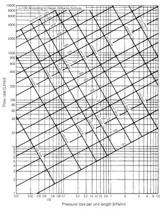
Fig. 25. Rigid vinyl chloride lined steel pipe flow rate diagram (SHASE-S 206-2009)
