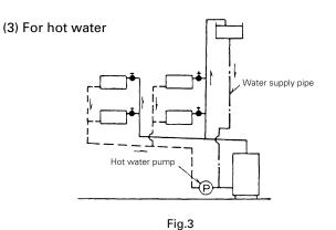
Used for circulating hot water between a heat source such as a boiler and a radiator.
