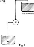
Used for pumping water from the receiving tank to the elevated tank.
