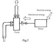
The energy that the motor rotates is called output or shaft power, and the energy causes the impeller to rotate and the pump to pump up water.
