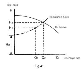
Selection of a pump in the selection diagram is just to find a pump with a Q-H curve through a single point (Q1, H1) determined by the pump discharge rate Q1 and total head H1 required at the calculated site.
