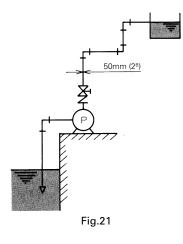
In the piping system shown on the left, the total frictional loss is calculated for a total length of 120m straight pipes with a pipe diameter of 50mm, one foot valve, four elbows, one check valve, and one gate valve. The volume of water conveyed shall be 0.2m<sup>3</sup>/min, and the pipes shall be carbon-steel pipes for pipes. Length of the straight tube... 120m
