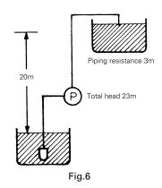
The pump must be capable of sucking water and discharging it, i.e. suction and discharge. The sum of the suction capacity and discharge capacity is defined as the pump's pumping capacity (pumping capacity), and is expressed as the total pump head in meters.
