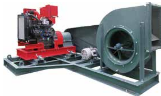
Sirocco fan (multi-blade fan) engine & motor driven, single inlet belt driven straddle mounted impeller type CLF2 (R) -RS-Y
