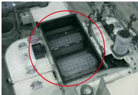
Drum filter is easily replaced.
